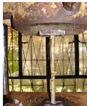
Fig.10 Bamboo sample Under Tension
