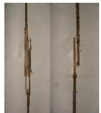
Fig.11 Typical tensile failure at knot between grip.
