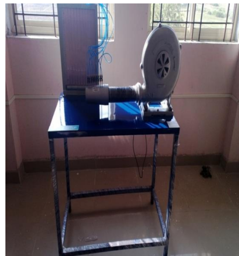
Figure 1; Convergent Nozzle experimental Setup
