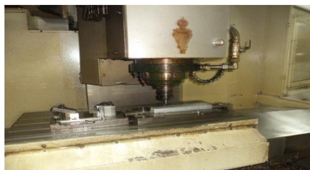
Fig 2. Shows the friction drilling setup on vertical CNC milling machine.
