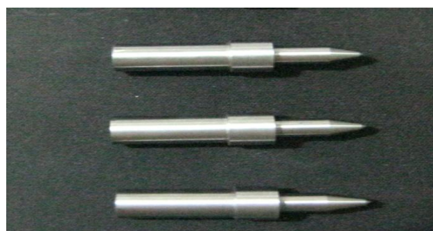
Fig 3. shows the Friction drills made up of HSS
