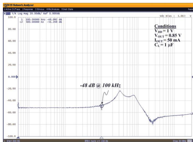
Fig. 7. Measured PSR performance. ( V_{DD}/V_{OUT}/I_{OUT} = 1 V/0.85 V/ 50 mA).
