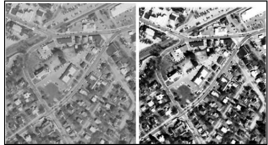
Fig. 2.3: Original Gray Image and Its Histogram Equalization Image
