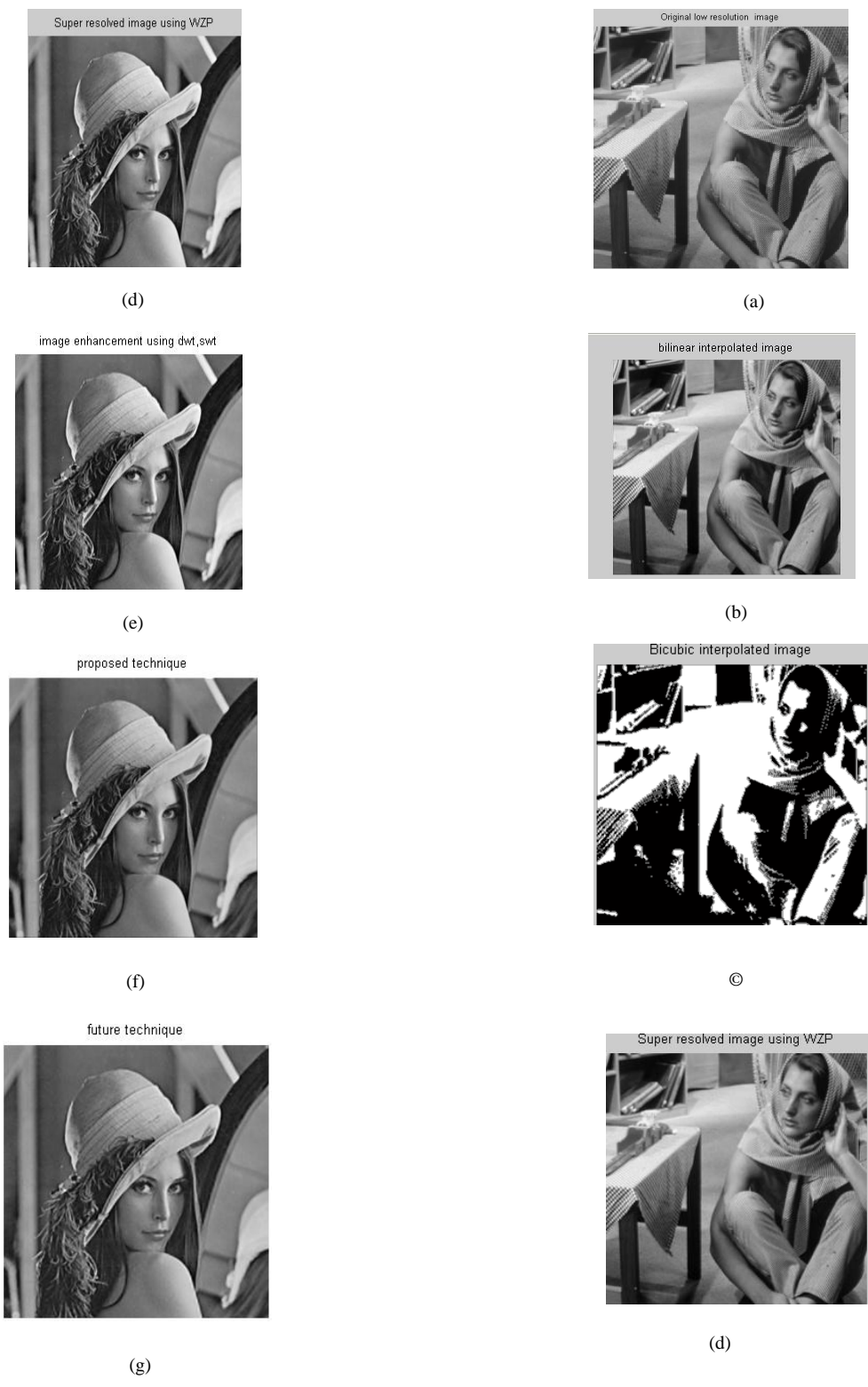
Fig. 4: Results for Lena Image (a) Low-resolution image obtained from down sampling of the high-resolution satellite image through two cascaded DWT, (b)Bilinear interpolation based resolution enhancement (c)Bicubic interpolation-based resolution enhancement, (d)Super resolved image using WZP, (e) Image resolution enhancement technique, using DWT and SWT (f) DWT based image resolution enhancement (g)Super resolution image using DWT and spatial domain input image
