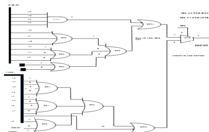
Fig 5.14 Internal structure of Input Output decoder
