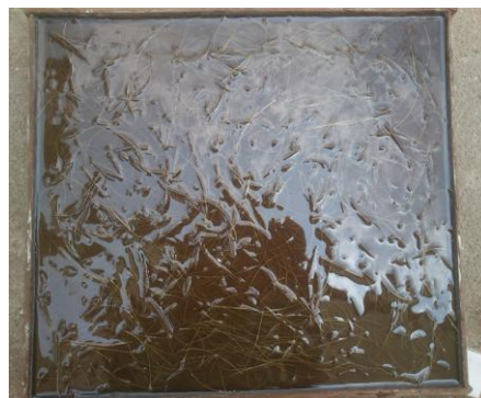
Fig. 2: Spreading coir on vinyl ester
