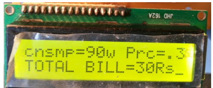
Fig.4 LCD output at customer house
