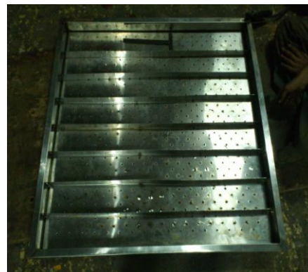
Fig. 4 Actual photo of adsorbent bed
