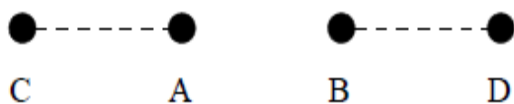
Figure 5 Neighboring nodes A and B have different schedules. They synchronize with node C and D respectively
