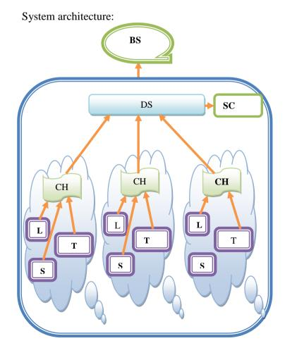
S->smoke, BS-> base station, S-> secure count, DA->data aggregation, T->temperature, CH->cluster head, L->light
