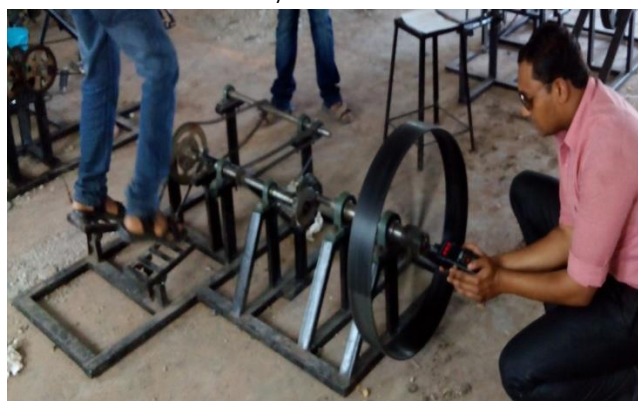
Figure 4. Practical model of double lever inversion in flywheel motor
