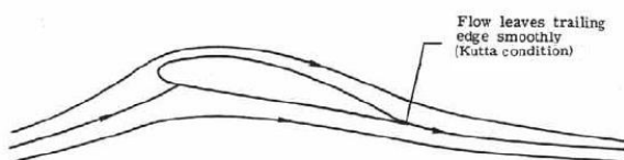
Fig. 2 Kutta condition applied
