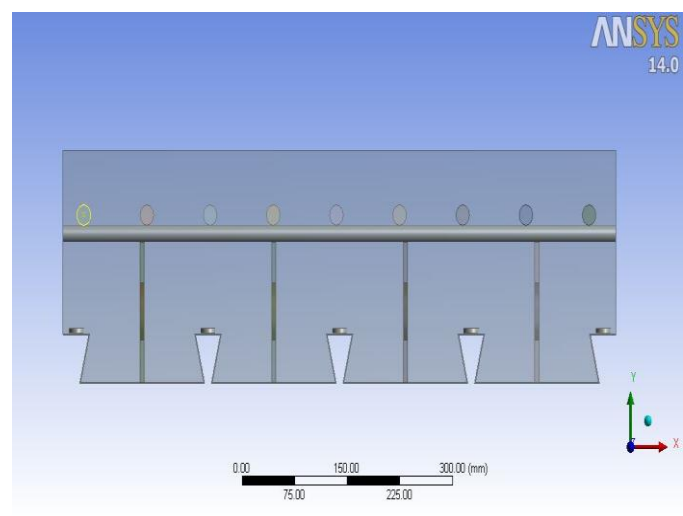
Fig. 7 Cross-section of Holorib profile sheet
