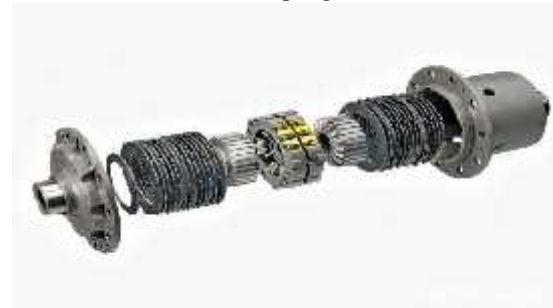
Fig.4.1 Clutch Type Limited Slip Differential
