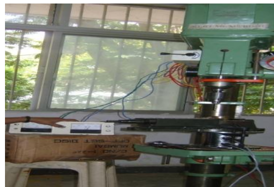
Fig1: Setup of drill tool dynamo meter
