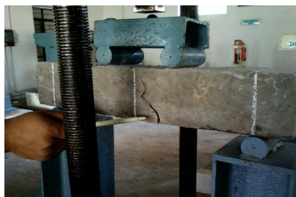
Figure 10 Failure of rubberised Concrete beam
