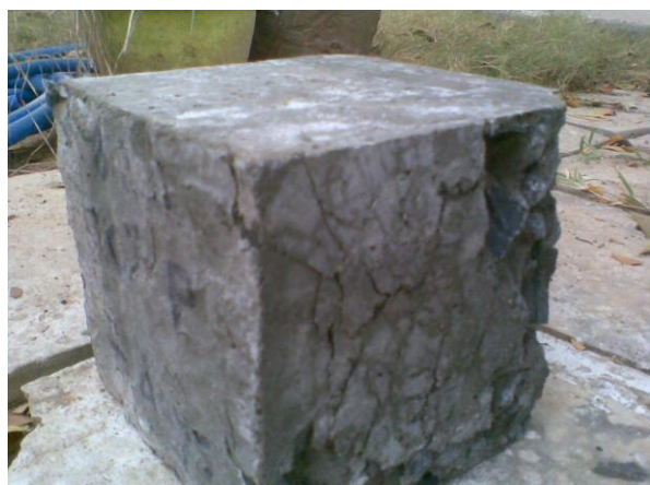
Figure 4 Rubberised Cube after Compressive Test
