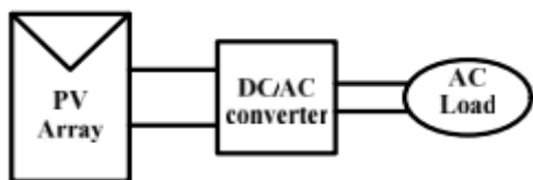
Fig.6. Block diagram representation of Photovoltaic system
