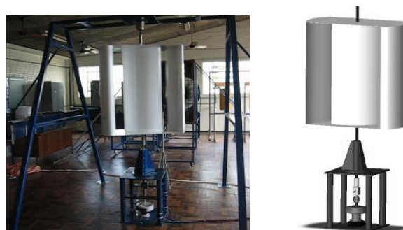
Figure 1 – New concepts of vertical axis small wind turbines for battery charging applications
