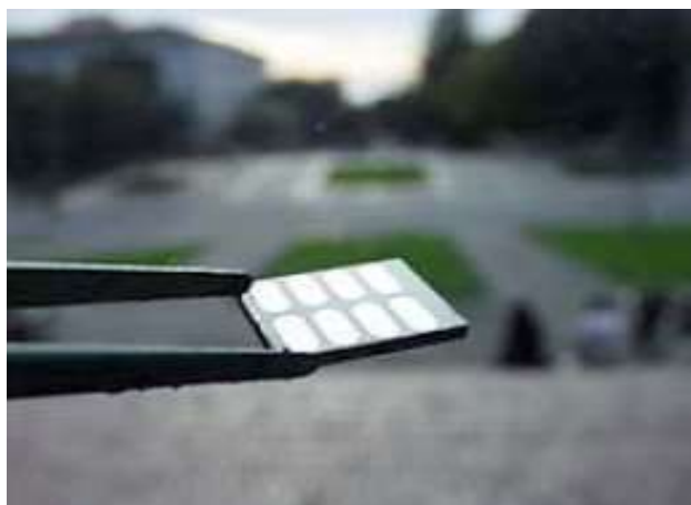
Fig.11 Solar cell utilizes nanorods to convert light into electricity [1]
