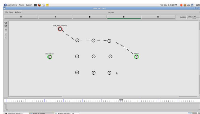
Fig. Packet transmission at the time of Sinkhole attack.
