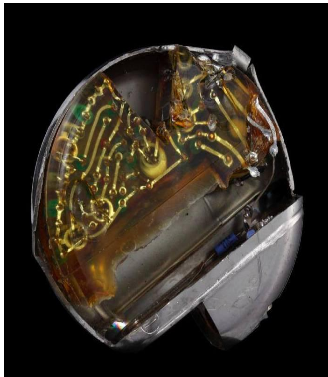
Fig.1 Internal structure of pacemaker
