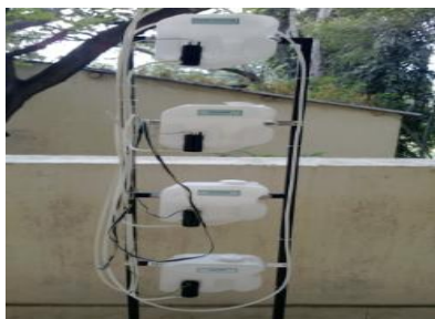
Figure 9: water and pesticide dosing, sprinkling tanks with dc sprinkler motors
