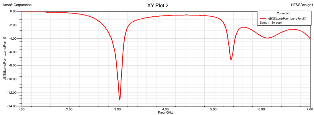
Figure 4: Simulated return loss [S11]
