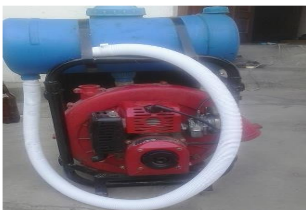
Fig.2 Fabricated model of pneumatic picking machine.
