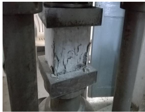
CUBE COMPRESSIVE STRENGTH TEST AFTER TESTING
