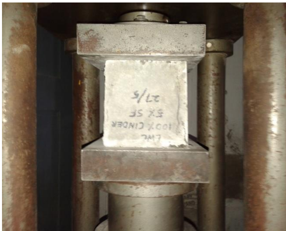
CUBE COMPRESSIVE STRENGTH TEST BEFORE TESTING
