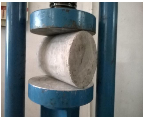
SPLIT TENSILE STRENGTH TEST BEFORE TESTING
