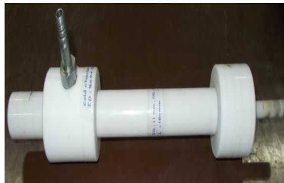
figure :2.vortex tube with PTFE Teflon material.
