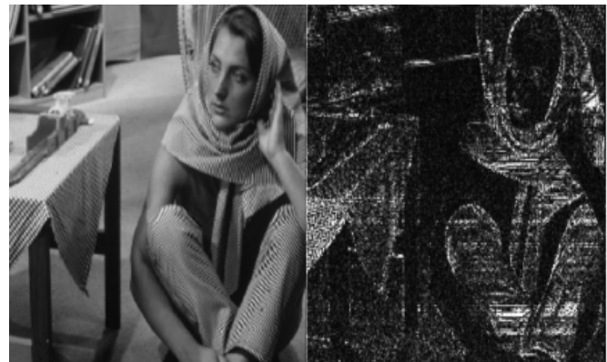
Fig. 6. Coefficient magnitudes of (top) JPEG 2000 and (bottom) ADL after one level of decomposition.
