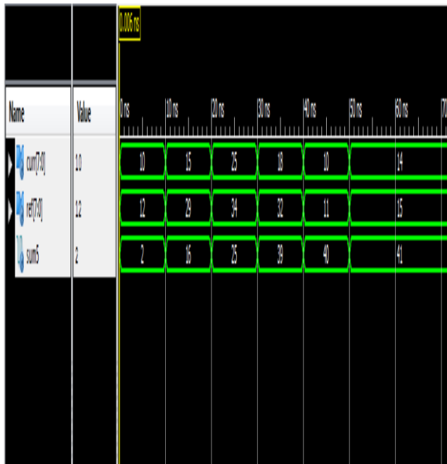
Fig 5: Simulation Waveform for Absolute difference
