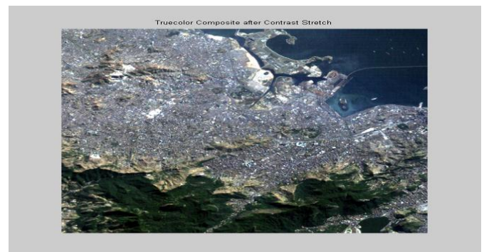
Figure 4. Result of contrast stretching on satellite image
