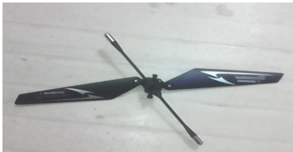
Fig.3.Upper Rotor Blade along with stabiliser Bar
