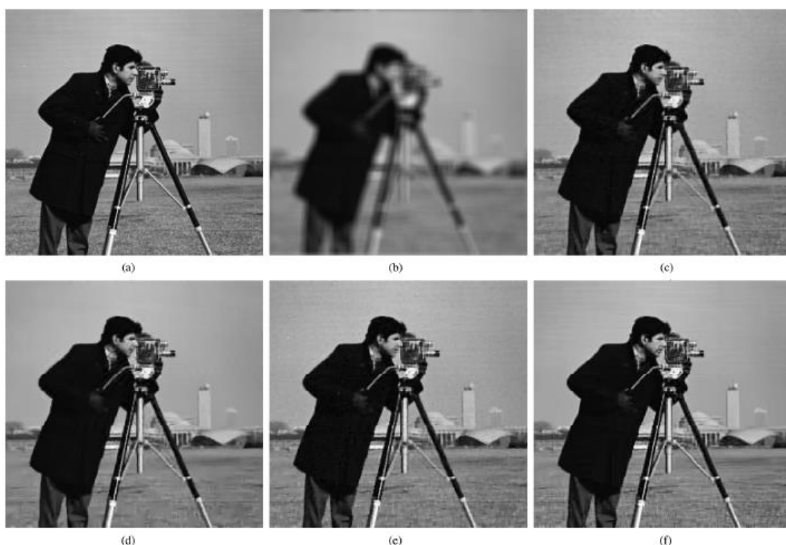
Fig. 5 comparison of original cameraman images, noisy blurred image (BSNR = 40 dB, 9 \times 9 uniform blur) and deblurred images by different algorithms); a) Original image; b) Noisy blurred image; c) TVMM (ISNR = 8.48 dB); d) SADCT (ISNR = 8.57 dB); e) IST ( ISNR = 8.65 dB) ; f) fine-granularity and spatail-adaptive regularization (ISNR = 9.96 dB).
