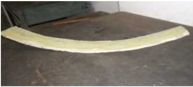
Fig. 2 Final trimmed composite mono leaf spring
