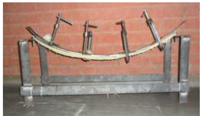
Fig. 1 Mould set up of composite mono leaf spring
