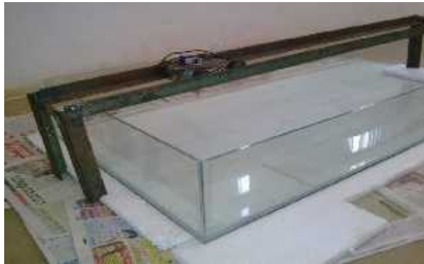
Fig: 1. Experimental Setup of surface visualization of vortex flows
