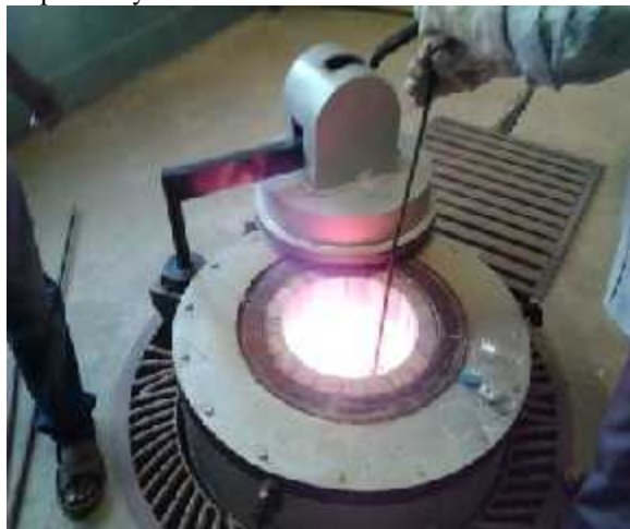
Fig. 1: Electric resistance furnace
