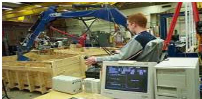
Fig.6 Tele-vator's Excavation Backhoe
