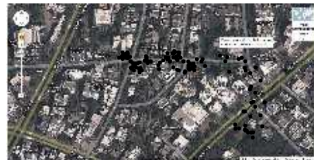
Figure 3 GPS data on map To obtain travel sequence, assign each cluster a unique ID, and substitute each point in the original chronologically ordered GPS trace with ID of the enclosing clusters.
