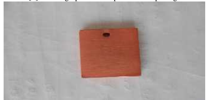
[4] Photograph 8: Work piece after plating This test is conducted on microscope by observing grain structure on plated metal.
