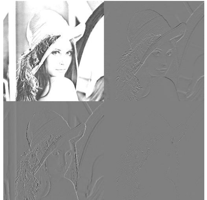
Figure 3.1 single level decomposition on lena image
