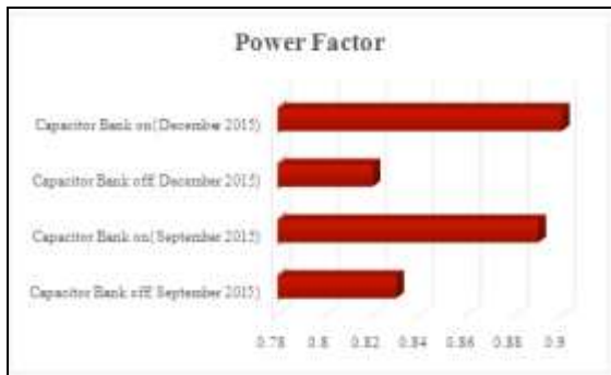
Figure 5.9 Power factor improvements
