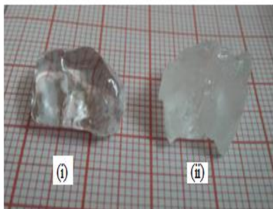
Fig.1. (a) Undoped hippuric acid crystal and (b) mercury chloride doped hippuric acid crystal
