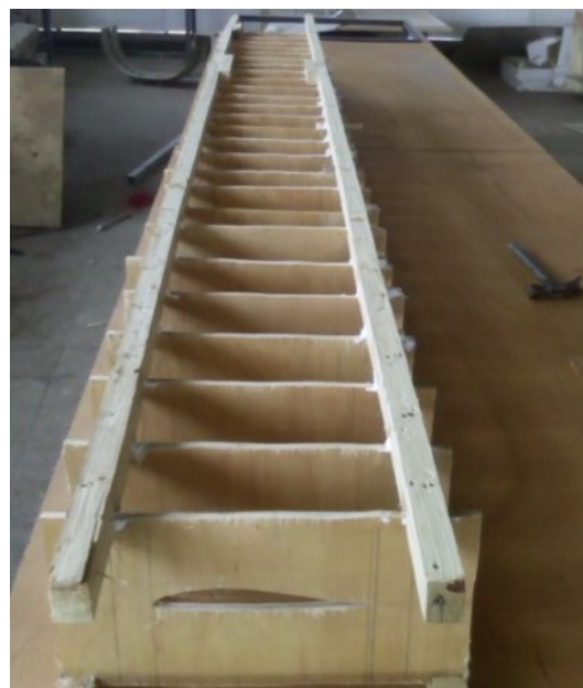
Step 7 Split the upper and lower part of airfoils
