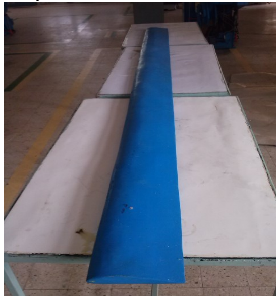
Step 21 Painting the parts using aviation grade paint and finalizing the surface finish for good aerodynamic task
