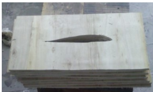
Step 4 Stacking all the airfoils on the prepared frames at equal interval of 135 mm
