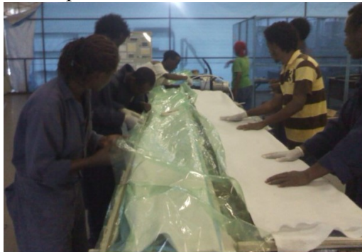
Step 18 Plugging vacuum pumps at both ends of the blade using T joint
