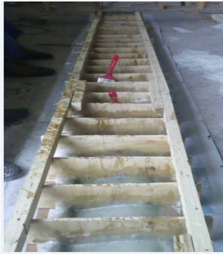
Step 11 Remove the cover sheet and smooth the surface using stucco
