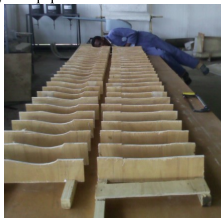
Step 8 Smoothing the surface of split molds using sand paper
