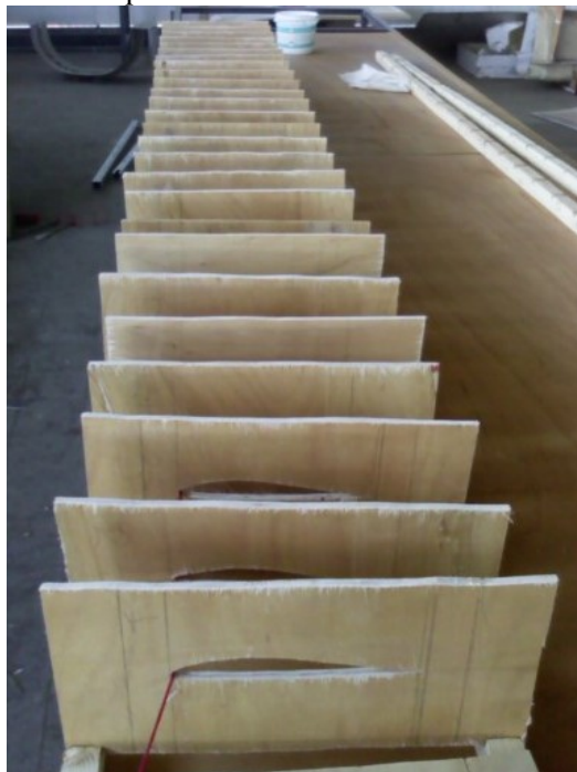
Step 4 Stacking all the airfoils on the prepared frames at equal interval of 135 mm
