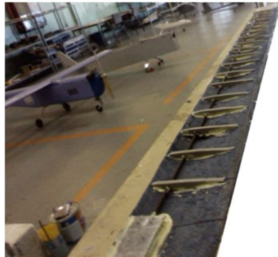
Step 20 Attaching the two halves using araldite, filler, and polyester resin
