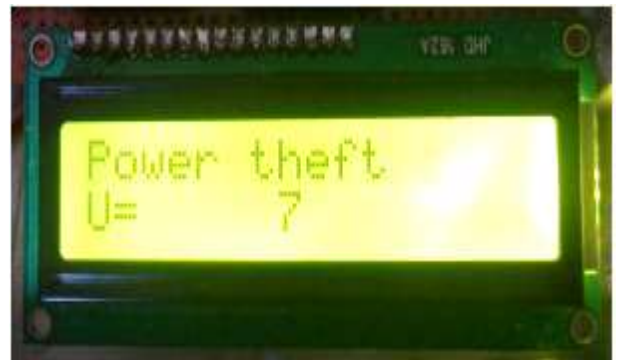
Fig 10:Display of power theft after consuming certain units
