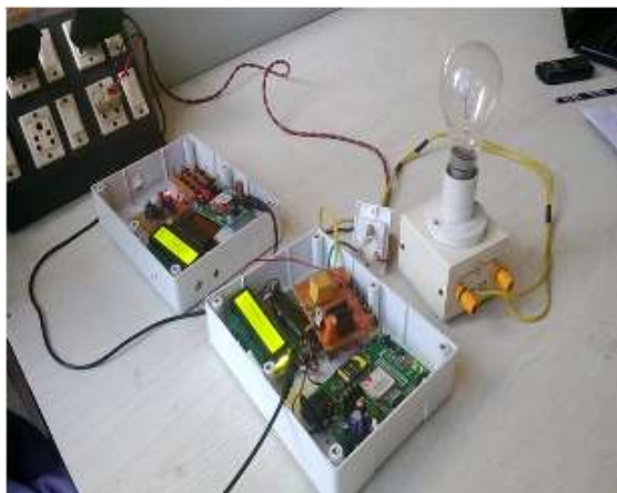
Fig 16: Relay open and no power to consumer detect illegal electricity consumption, by GSM based
