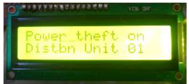
Fig 11:Display of power theft from particular distribution unit
