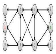
Destination. Each node has a routing table and updates its routing table regularly. Also, they exchange RIP (Routing Information Protocol) every 60 seconds and after 180 seconds, if no response is detected, they regard as it is notconnected1.
