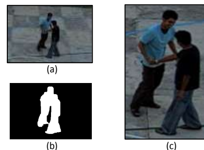
Fig7: (a) Original Frame (b) Motion Segmentation (c) Resized Region of Interest
