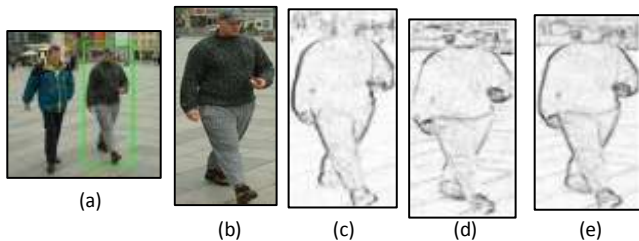
Fig 4: (a) Original Image with Bounding Box and Resized Image. (b) Resized Image (c) Horizontal Gradient (d) Vertical Gradient (e) L1 Normalized Gradient
