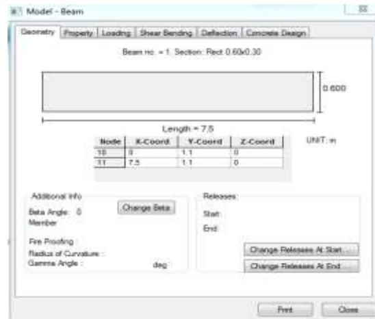
Fig 1: Geometry of beam no.1
