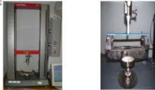
Figure – 17 (a) UTM testing machine (b) Specimen in jaws Three point flexural test Three point bending tests of specimen were carried out in using Zwick/Roell (Figure – 17 & Figure - 18).
