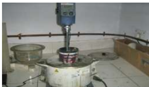
Figure – 7 Oil bath setup with mechanical stirrer
