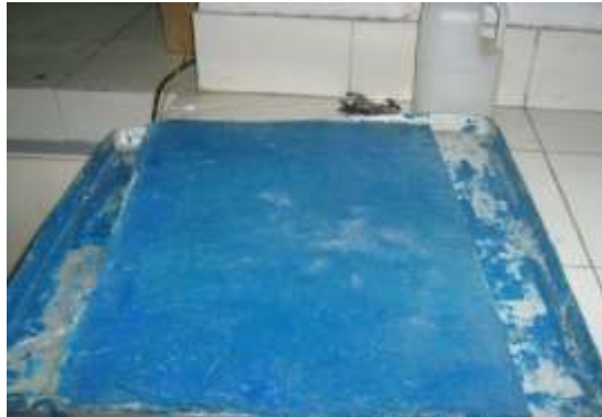
Figure – 11 Coated sheets placed for curing
