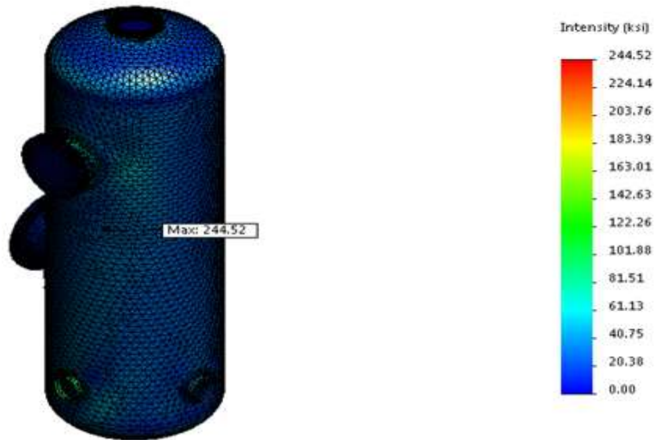
Figure - 9 Von Misses distribution comparison
