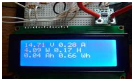
Fig.2 module of smart energy meter displaying power consumption.
